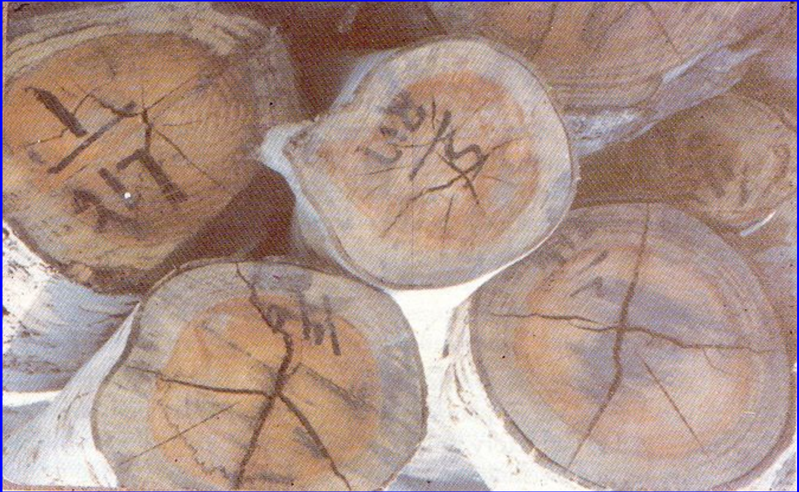
Eucalyptus with end cracks
