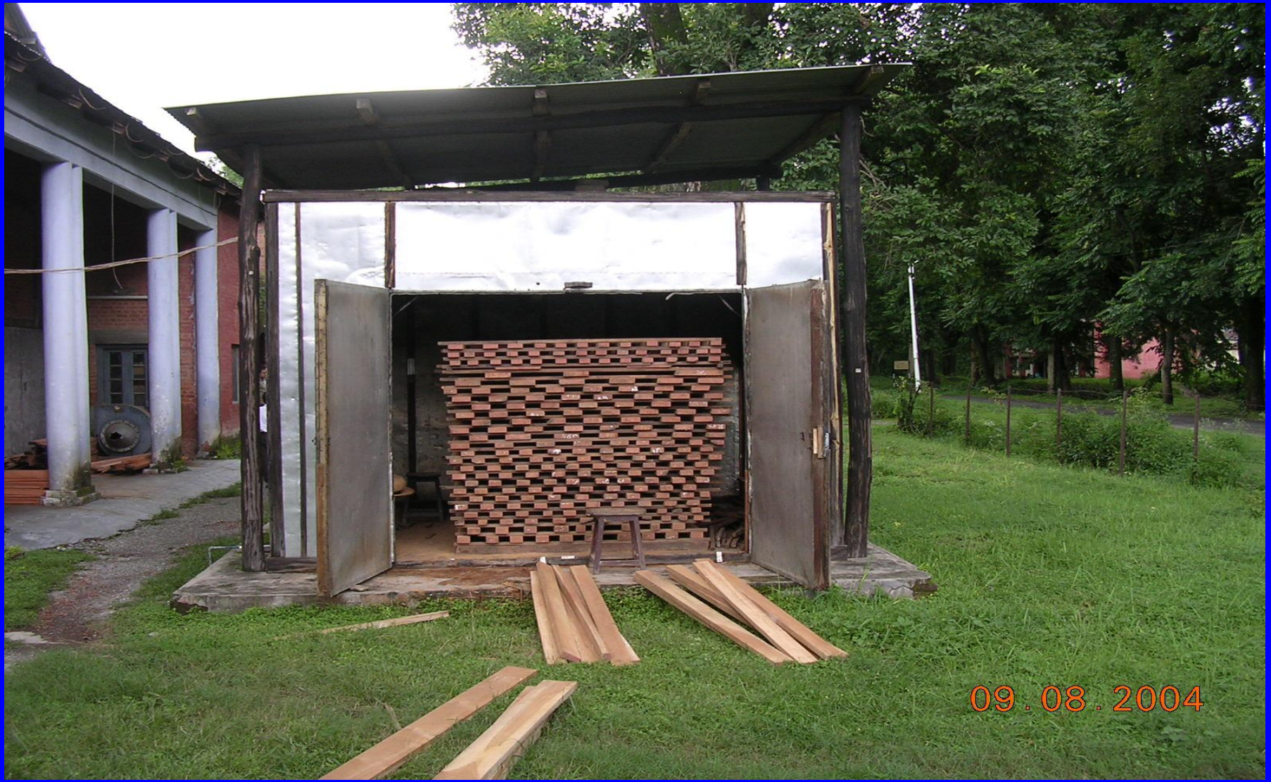
Wood stack loaded inside an Electrical Kiln
