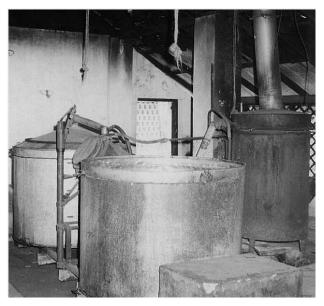
**Retort**: Retort or still proper commonly called as 'tank' serves primarily as a container for plant material and as a vessel in which water and or steam contacts plant material and vaporizes its essential oil.
