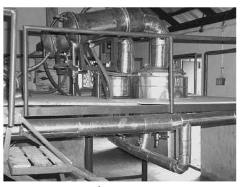
Solution is subsequently pumped into an evaporator and concentrated at a low temperature. After the solvent is completely driven off in vacuum, concentrated flower oil is obtained. Thus, temperature applied during entire process is kept at a minimum; live steam as in case of distillation, does not exert its action upon delicate constituents of flower oil. Compared with distilled oils, extracted flower oils more truly represent natural perfume as originally present in flowers.
