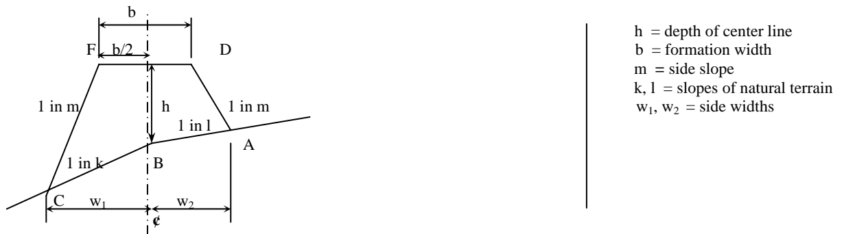
Fig 7.18 : Embankment ( Three Level Section )
