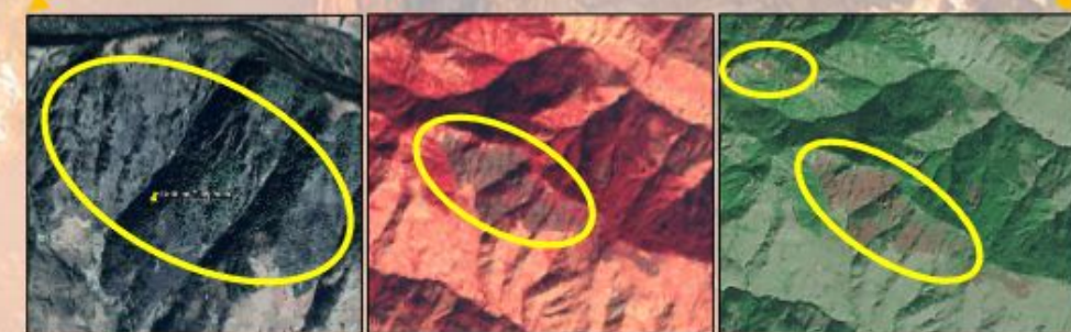
Google Earth Image: 27.11.2016 Landsat-8 OLI Image: 06.12.2016 Sentinel-2A Image: 11.12.2016 Imagery of different satellites showing the burnt scars representing the winter fires starting from week no 47 (19th November to 25th November 2016)
