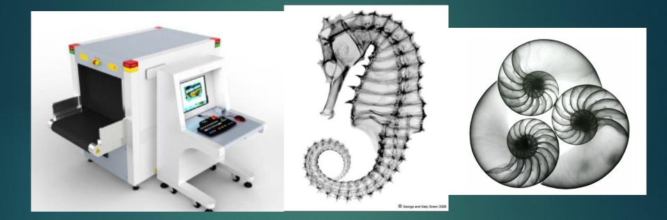
X-Ray Scanners at the transit areas are placed to scan baggage's to detect any contraband in transit
