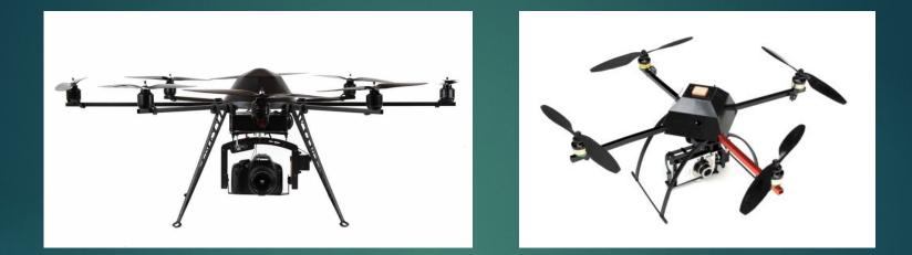
Mikrokopters are universal aerial platforms that hover. They can identify a position and hold it as long as necessary to identify images, collect data, or calculate distances. They are equipped with GPS, compasses, altitude control, telemetry
