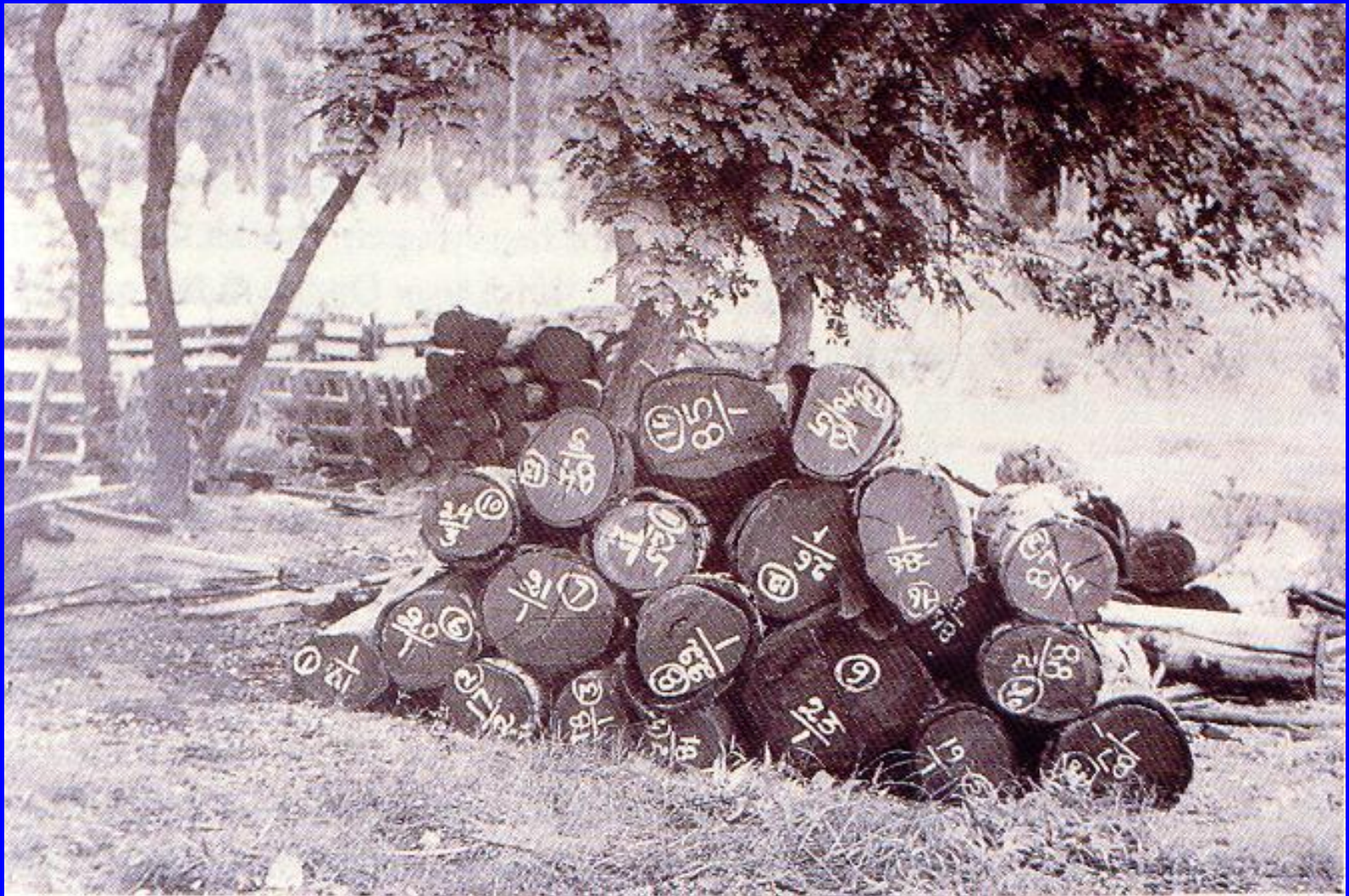
End coating for controlling end cracking in Eucalyptus
