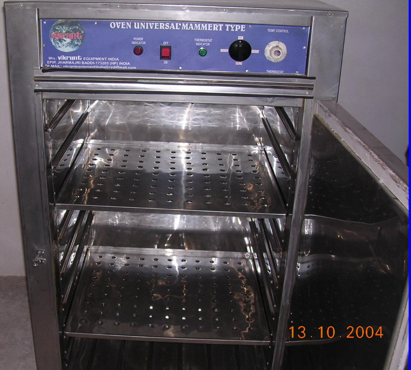
A laboratory oven used for determining moisture content in wood samples
