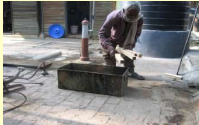
Preservative application through dipping/soaking
