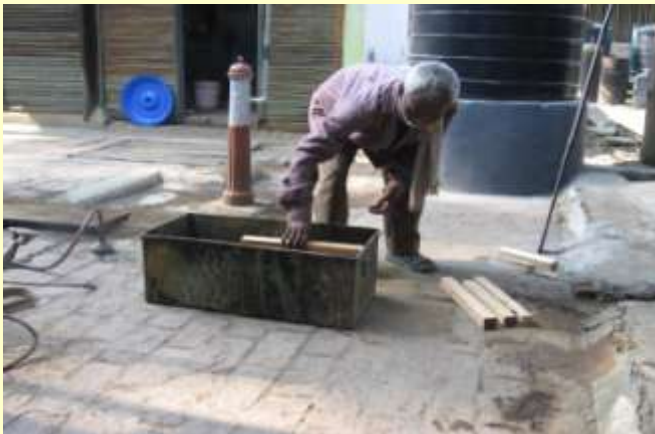
Preservative application through dipping/soaking
