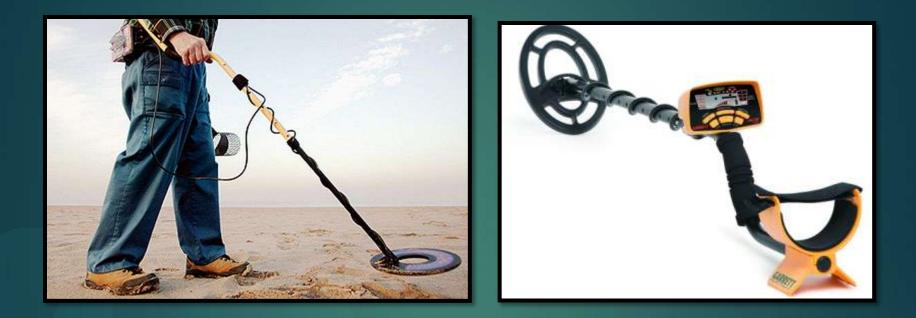
Metal Detectors used in the protected areas help locating leg hold traps and wire snares fixed by poachers.
