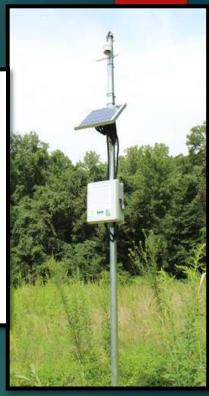
Acoustic Traps use "echo technology" to monitor sharp disturbances such as gun shots, chain saws, truck engines, blasts etc. using monolithic sensors.
