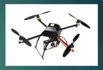
Mikrokopters are universal aerial platforms that hover. They can identify a position and hold it as long as necessary to identify images, collect data, or calculate distances. They are equipped with GPS, compasses, altitude control, telemetry
